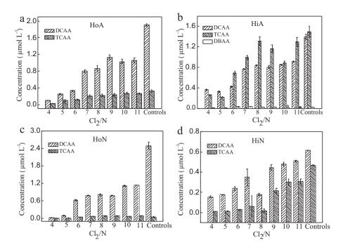
**Fig. 6.** Effect of Cl<sub>2</sub>/N ratios on the formation of HAAs. HoA, hydrophobic acids; HiA, hydrophilic acids; HoN, hydrophobic neutrals; HiN, hydrophilic neutrals; Controls, samples without addition of NH<sub>3</sub>–N. All samples were conditioned to similar DOC concentrations of about 3 mg/L. The experimental conditions were pH=7.0; chlorine dosage = 20 mg/L as Cl<sub>2</sub>; temperature = 20 °C; and contact time = 3 days.
