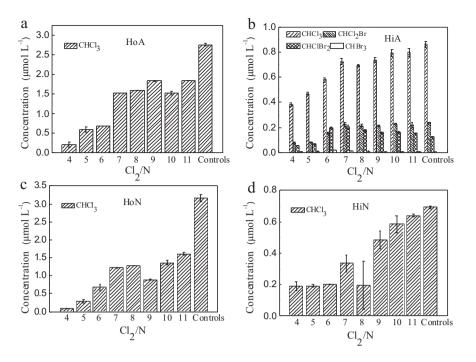
**Fig. 4.** Effect of Cl<sub>2</sub>/N ratios on the formation of THMs. HoA, hydrophobic acids; HiA, hydrophilic acids; HoN, hydrophobic neutrals; HiN, hydrophilic neutrals; Controls, samples without addition of NH<sub>3</sub>–N. All samples were conditioned to similar DOC concentrations of about 3 mg/L. The experimental conditions were pH=7.0; chlorine dosage = 20 mg/L as Cl<sub>2</sub>; temperature = 20°C; and contact time = 3 days.
