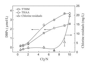
**Fig. 1.** Chlorine residuals and DBP formation of the effluent at different  $Cl_2/N$  mass ratios. Experimental conditions were DOC = 7.2–8.2 mg/L; pH = 7.0; NH<sub>3</sub>–N concentration = 3.0 mg/L as N; temperature = 20 °C; and contact time = 3 days.
