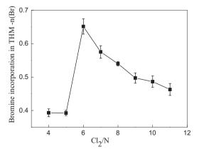
Fig. 5. Bromine incorporation in THMs as a function of Cl<sub>2</sub>/N mass ratios of the HiA fraction. HiA, hydrophilic acids.
