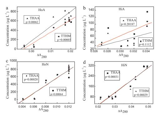
**Fig. 7.** The relationship between  $A_{280}$  loss ( $\Delta A_{280}$ ) and the formation of DBPs. HoA, hydrophobic acids; HiA, hydrophilic acids; HoN, hydrophobic neutrals; HiN, hydrophilic neutrals. All samples were conditioned to similar DOC concentrations of about 3 mg/L.
