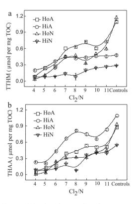
**Fig. 3.** Chlorine residuals and DBP formation of DOM fractions at various  $Cl_2/N$  ratios. HoA, hydrophobic acids; HiA, hydrophilic acids; HoN, hydrophobic neutrals; HiN, hydrophilic neutrals; Controls, samples without addition of  $NH_3-N$ . All samples were conditioned to similar DOC concentrations of about 3 mg/L. The experimental conditions were pH = 7.0; chlorine dosage = 20 mg/L as  $Cl_2$ ; temperature =  $20^{\circ}C$ ; and contact time = 3 days.
